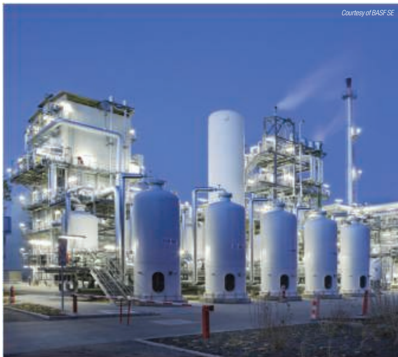
FIGURE 4. Most PSA systems, such as the one shown here, are used for separating hydrogen from a gas mixture
