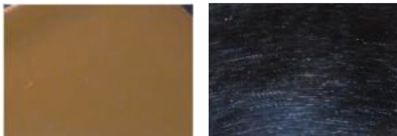
FIGURE 3. Figure 3a (left): A stainless steel surface viewed under diffused light appears pristine. Figure 3b (right): By contrast, the same stainless steel surface, viewed under undiffused light, reveals surface imperfections that may or may not be significant
